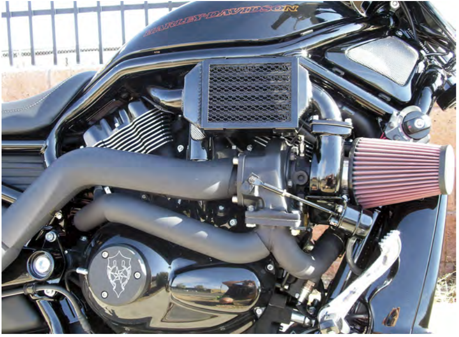
2008 Nightrod Custom 1250 stock V-Rod Engine. Trask Intercooled Turbo System 8.0lbs of boost, 91 octane pump Gas, SE Race Tuner.
