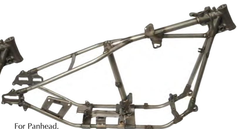
For Panhead. Model year 1954 with neck 30° "Wishbone" With German TÜV certificate Individual requests are possible
