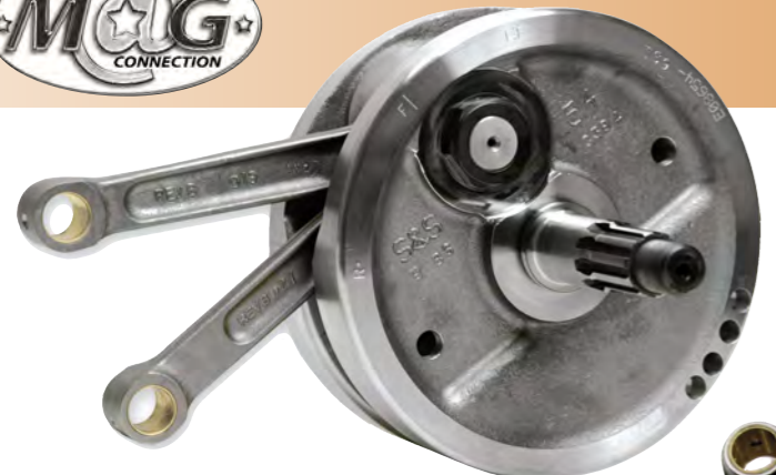
Flywheel Assembly with 4-5/8\" Stroke Assembly is for 1973-1984 Big Twin and are machined from heat treated steel forgings. Cover features natural cast finish, as original!
