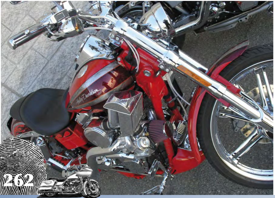
2008 SE Dyna Stock TC 1100" w/ SE 255 Cams. Trask Intercooled Turbo System 8.0lbs of boost on 91 octane pump gas. Thundermax Auto Tune
