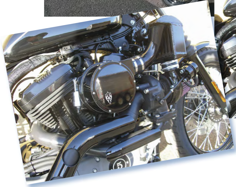
2008 Nightrod Custom 1250 stock V-Rod Engine. Trask Intercooled Turbo System 8.0lbs of boost, 91 octane pump Gas, SE Race Tuner.
